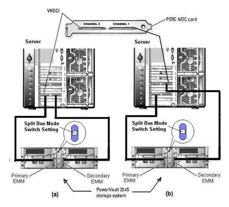
Figure 4-3 Split Bus Cabling Options to a Single Host System, (a) Same Adapter, (b) Different Adapters
