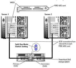
Figure 4-2 Split Bus Cabling to Two Host System
