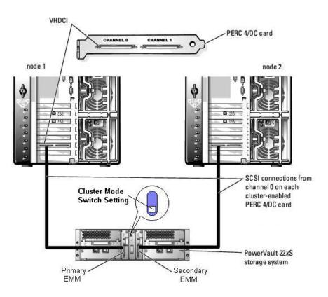
Figure 4-4 Cluster Topology Cabling Example
